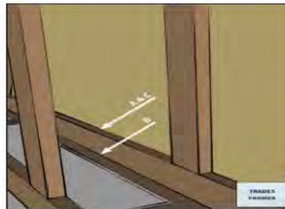
Air seal the common wall between units in a multi-family structure to minimize air leakage.
