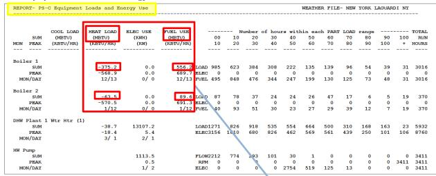
WHVAC03, WHVAC14: The average realized plant (boiler or chiller) efficiency is the ratio of Heat Load to Fuel Use. In the example, the average efficiency of the Hot Water Plant (Boiler 1 and Boiler 2 combined) is 68%.
