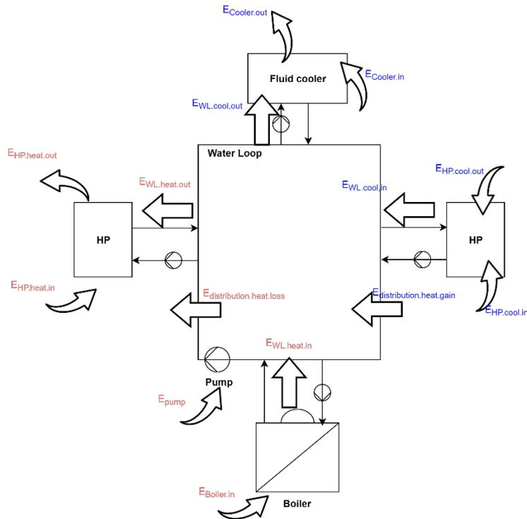
Figure 65. Schematic diagram of Water Loop Heat Pump
