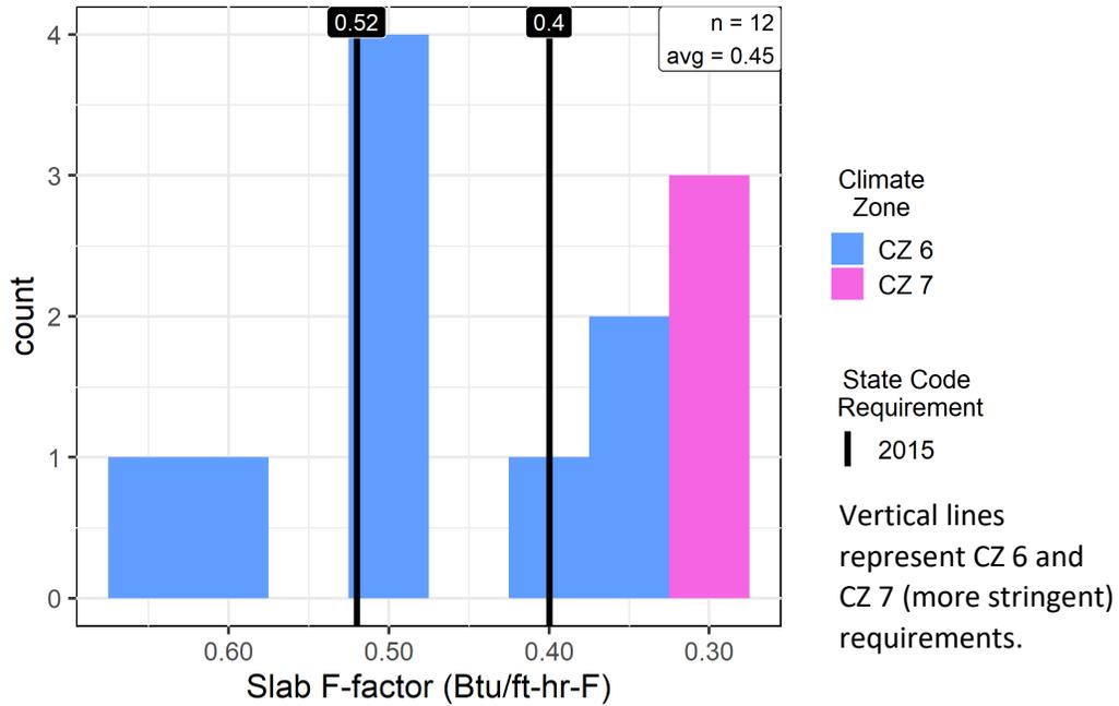
Figure 15. Minnesota Slab F-factor
