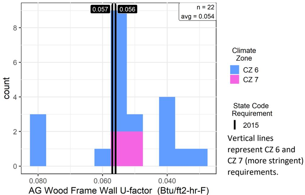
**Figure 14. Minnesota Above Grade Wall U-factor (Wood-Frame Walls)**
