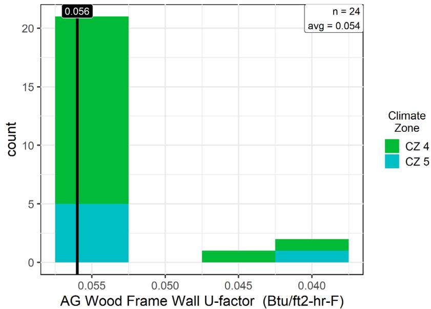
**Figure 27. Washington Above Grade Wall U-factor (Wood-Frame Walls)**
