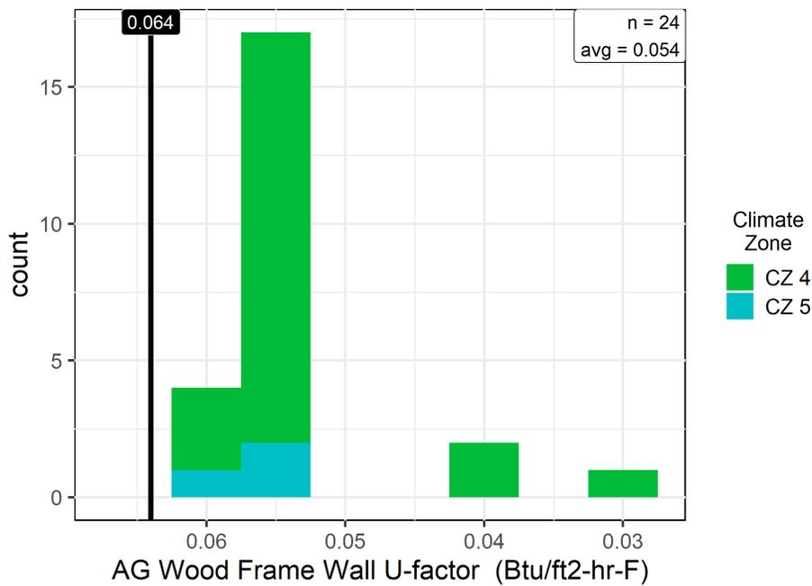
**Figure 21. Oregon Above Grade Wall U-factor (Wood-Frame Walls)**
