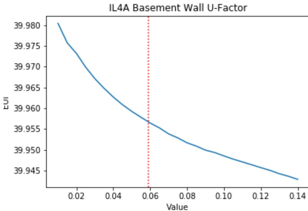
Figure 67. Illinois 4A Basement Wall U-Factor
