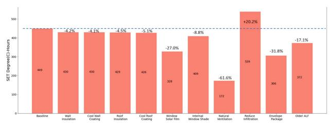
Figure 15. Average SET Degree Hours (above 86°F) of the Baseline and Improved Assisted Living Facility Models with Passive Measures for the 2015 Heatwave
