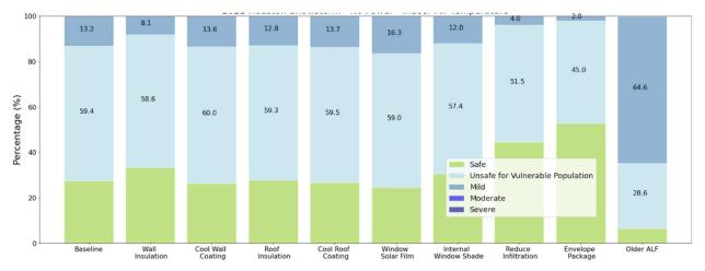
Figure 17. Percentage of Hours at Each Cold Stress Level of the Baseline and Mitigated Assisted Living Facilities with Passive Measures During the 2021 Snowstorm
