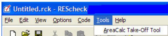
AreaCalc Take-Off Tool - This option launches the AreaCalc software tool that can be used to do building take-offs. The areas computed in AreaCalc can be transferred directly to REScheck.
