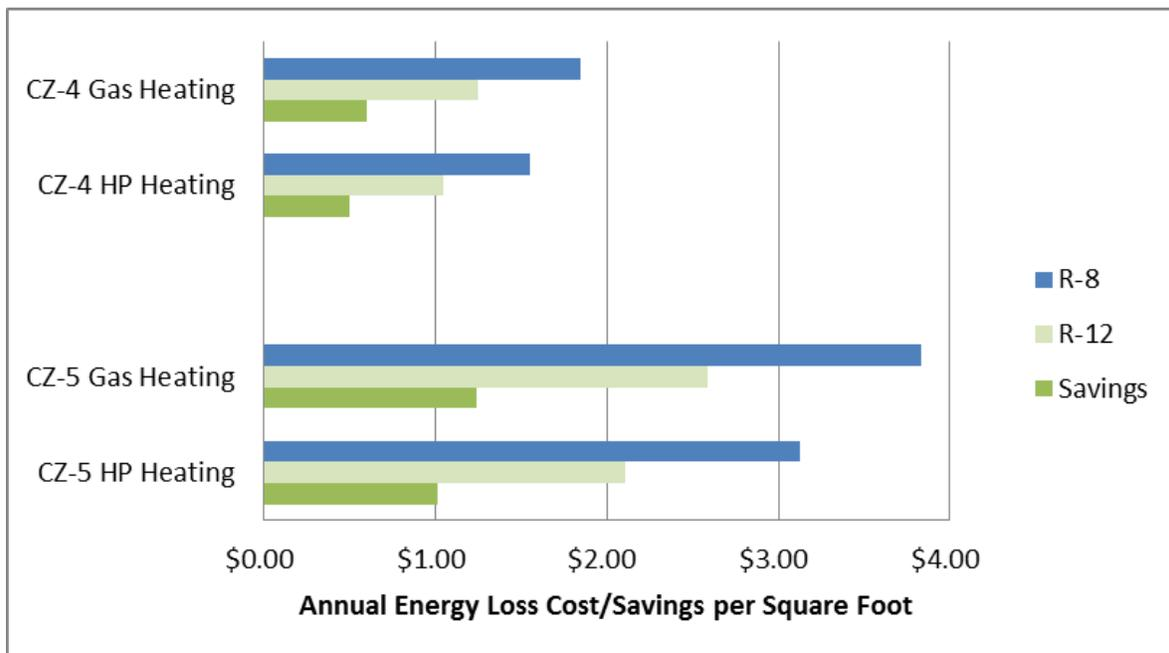
**Figure 1: Exterior Ductwork Annual Loss Cost and Savings**
