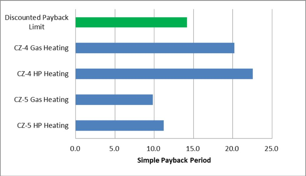
**Figure 3: Simple Payback for Added Duct Insulation**
